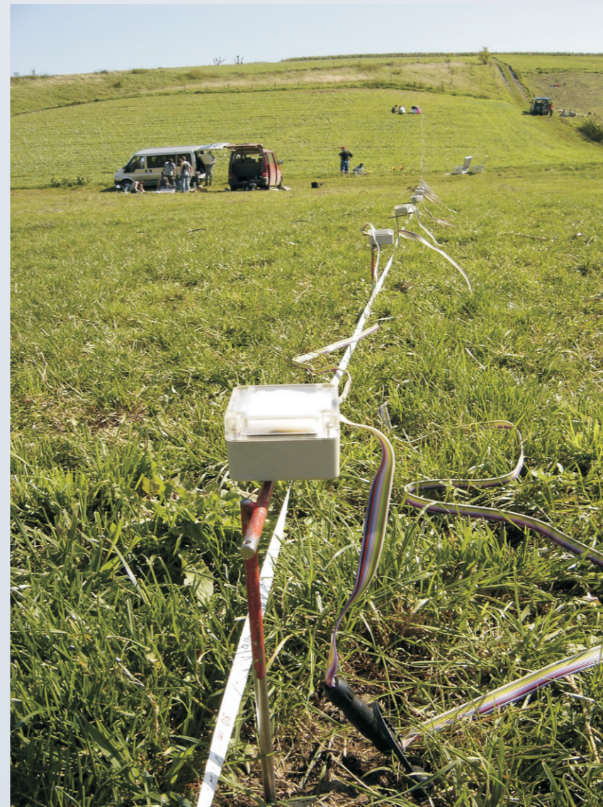
Electrode layout in field.
